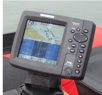
Seasearch East has used a small sidescan sonar to aid in the location of chalk exposures. The unit has an integrated GPS receiver for recording track, site and scan position. Interpreting sidescan sonar images is something of a black art which the team has been learning. The unit aims to provide a guide to substrate composition and density by colour coding a conventional sonar plot of the bottom but the trained human eye can be much more effective at interpreting information.
