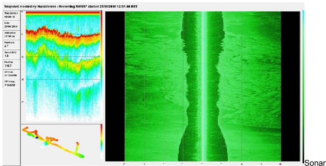
Sonar recording: Showing conventional sounding display (top left), track colour coded by depth (bottom left) and joined left and right side scans as the boat crosses a 1.5m ridge of chalk (right)
